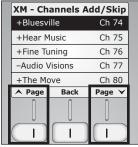
To scroll through channels within a page, press the **Cursor**A or **Keys**.
